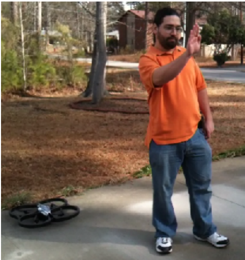
Figure 2: The initial implementation, here used to launch and land a drone, was based on a correlation threshold between a supplied signal (a “beat”) and perceived motion.
