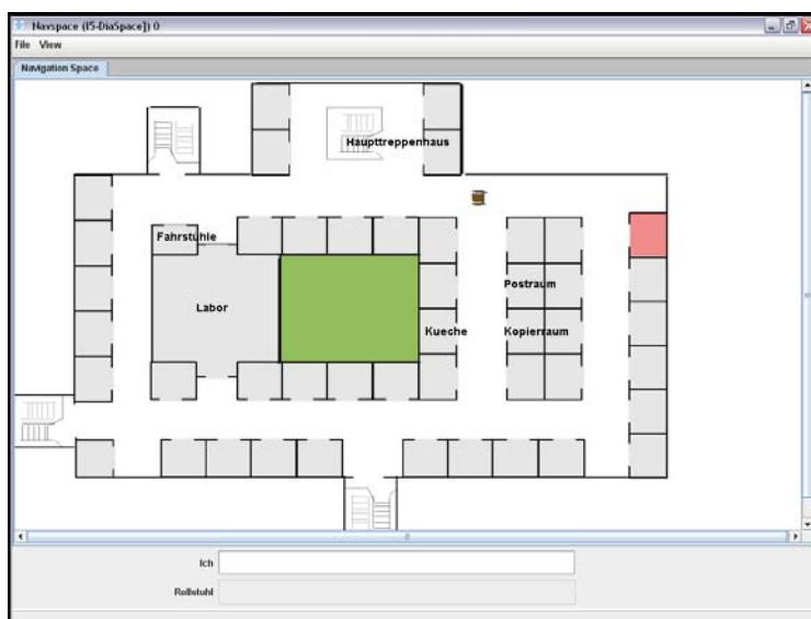
Figure 1. Our map instruction scenario. The robot wheelchair is indicated on the top hallway, facing towards the left side of the picture. The goal location is marked for the instruction giver only; the location labels are always visible. In the HHI case, joystick movements by the instruction receiver make the wheelchair move on the screen; in the HCI case, the wheelchair movements are handled by the system.
