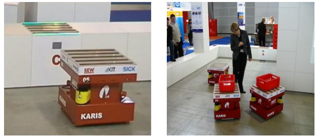
Figure 2: The target system: Robots equipped with conveyor and RFID reader for autonomously handling transportation tasks: (a) approaching a station for loading. (b) safe navigation among humans.
