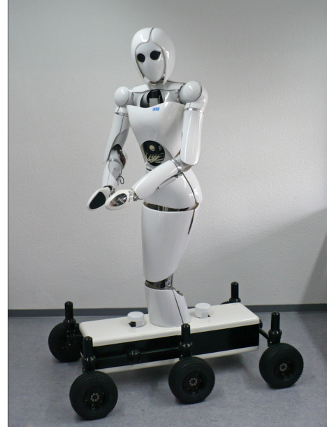
Figure 2. The semi-humanoid robot Aila, which was developed for dual manipulation tasks in a logistic scenario. The robot uses a tilting 3D LIDAR system for precise point cloud generation in 3D space. A second PMD LIDAR is used for obstacle avoidance.
