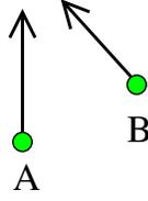
**Figure 2:** Qualitative spatial relation between two oriented points at different positions. The qualitative spatial relation depicted here is *A RightLeft B* (which reads: *B* is to the right of *A*, and *A* is to the left of *B*).
