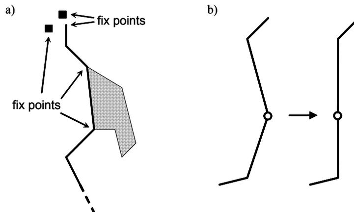
**Figure 1.** a) Examples of fix points: Single-point objects, endpoints of lines, and points shared by two or more objects are treated as fix points in the simplification process; b) Example of a simplification step: movable points on linear entities are projected back onto the entity after the simplification step
