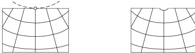
Fig. 3. Two Maps: The left map cannot contain a north grid line since the possible candidate for the north grid line shares only a single point with the map. The right map is a corresponding formal map including a north grid line
